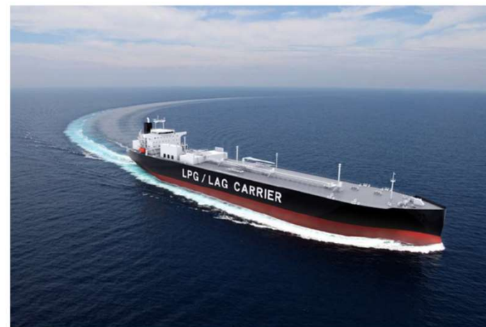
Image of an LPG-powered VLGC convertible to ammonia fuel
