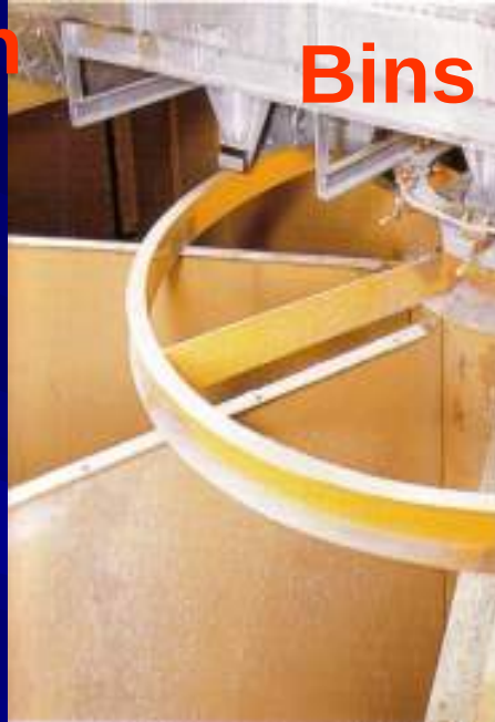
Round Silo on Top of Batching Plant with 5-6 Bins
